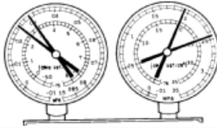
HINT : These gauge indications are shown when the refrigeration system has been opened and the refrigerant charged without vacuum purging.
